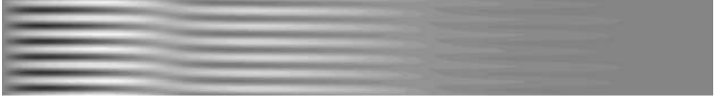
FIGURE 12. Instantaneous contours of streamwise velocity fluctuation ( -0.3 \leq u \leq 0.3 ) evaluated at y/\delta_0 = 0.58 . The streamwise extent shown is 0.4 \times 10^5 \leq R_x \leq 2.4 \times 10^5 . The spanwise coordinate 0 \leq z \leq 8 is enlarged by a factor of 3. Inlet mode: \omega = 0.032 , k_y = \pi , k_z = 4.7 , \Theta = 32.5 .
