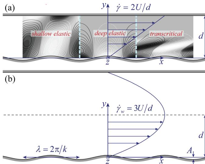
FIG. 1. (a) Schematic representation of Couette flow over a wavy surface, indicating the nature of vorticity perturbations predicted in the three regimes of viscoelastic flow [16]. (b) Schematic representation of Poiseuille flow over a wavy surface, as employed in the present study.
