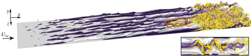
FIGURE 1. (Colour online) Visualization of a streaky boundary layer undergoing bypass transition. Light isosurfaces are high-speed streaks ( u' = 0.085 ) and dark surfaces are low-speed streaks ( u' = -0.085 ). Turbulence is visualized using isosurfaces of the \lambda_2 -criterion ( \lambda_2 = -0.005 ).
