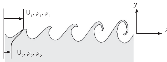
Fig. 1. Schematic of a two-fluid, incompressible mixing layer.
