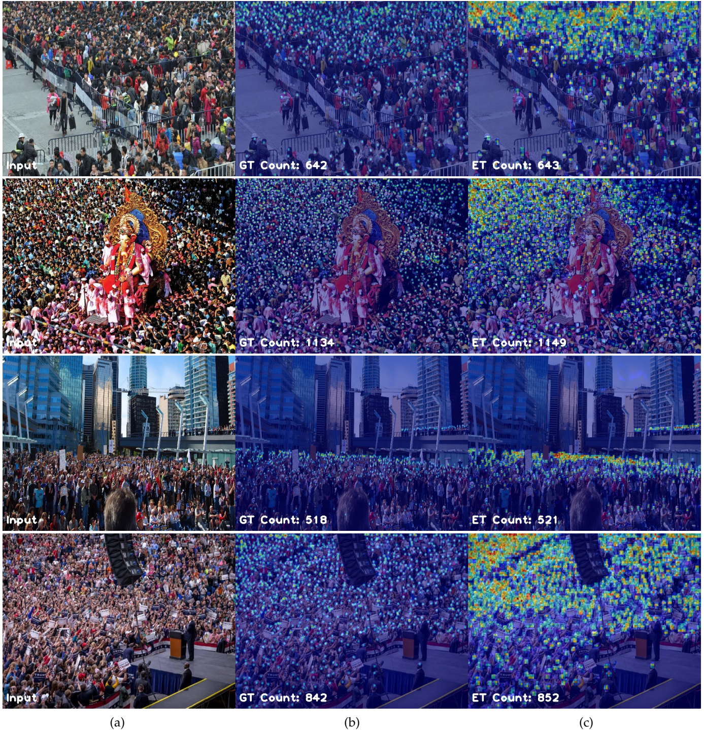
Fig. 13. Results of the proposed dataset on sample images from the JHU-CROWD++ dataset. (a) Input image (b) Ground-truth density map (c) Estimated density map.
