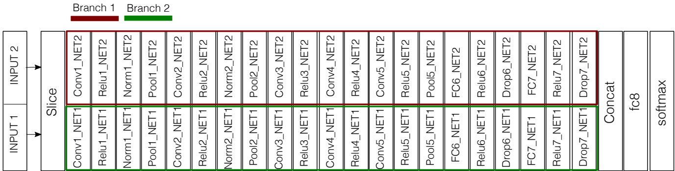
Fig. 3: CNN level fusion. The multimodal architecture for mmW Person Recognition with the Alexnet pre-trained model.
