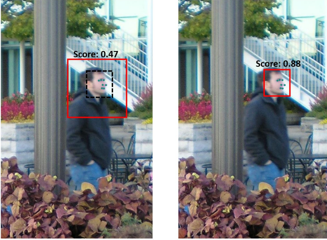
Fig. 3. Candidate face region (red box on left) obtained using Selective Search gives a low score for face detection, while landmarks are correctly localized. We generate a new face region (red box on right) using the landmarks information and feed it through the network to increase the detection score.
