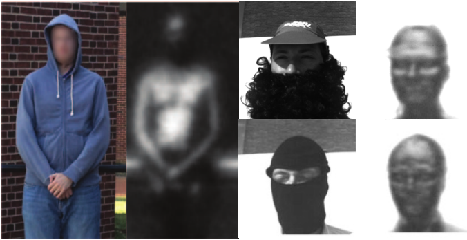
Fig. 2: Benefits of mmWs for imaging: i ) transparency through body clothes (extracted from [3], and ii ) transparency through face clutter (images from the mmW TNO database)
