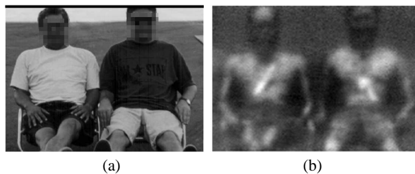
Fig. 1. Millimeter wave imaging through clothing. (a) Visible image of the scene. (b) Image produced using a 94-GHz imaging system.
