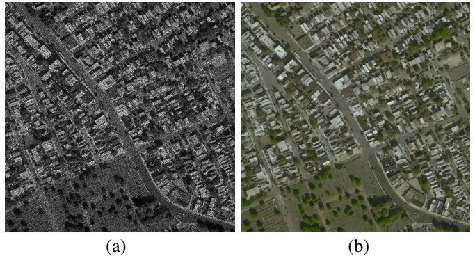
Fig. 1: A sample result of the proposed SAR-GAN method for SAR image to visible image translation. (a) Simulated input noisy SAR image. (b) Despeckled and colorized image.
