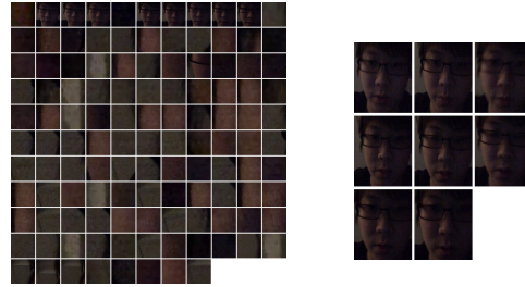
Fig. 3: Increasing the size of the smallest search window of VJ detector to 25% of the frame size eliminates all the false alarms within the 149 detections (shown in the left) made in a sample video file while keeping the 8 true positives (shown in the right).
