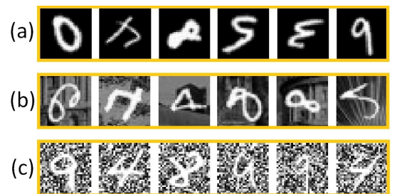
Fig. 4: Sample digits from the rotated MNIST dataset. (a) Digits with random rotations, (b) Digits with random rotations and image backgrounds, (c) Digits with random backgrounds.
