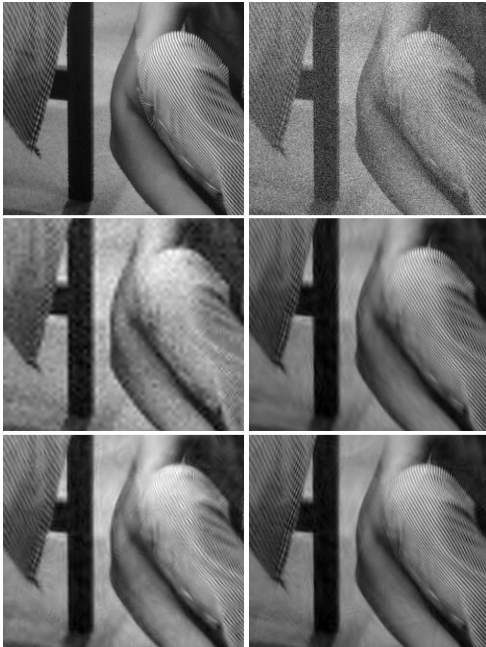
Figure 8. Close-up experimental results – From top left, clockwise: Original Image, Noisy image (PSNR= 22.12 dB), (BivShrink) using the Dual-tree Discrete Wavelet Transform (PSNR=29.72 dB), generalized Directional Filter Bank (PSNR= 29.97 dB), Curvelet Transform (PSNR= 26.58 dB), and Discrete Wavelet Transform defined in terms of the Daubechies-Antonini 7/9 filters (PSNR= 23.61 dB).
