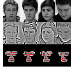
Fig. 2: The first row shows the original image before preprocessing. The second row is the image after illumination normalization. The final row demonstrates the facial landmarks and patches used in this work.
