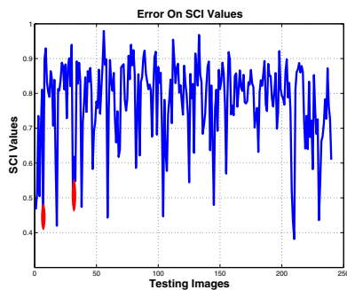
Fig. 8. Plot of the SCI Values of test images of a random trial of the ND dataset. Red dots indicate the wrongly classified images. Observe that the wrongly classified images have very low SCI values and hence the corresponding vectors are not sparse.
