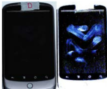
Fig. 1: Smudge attack [3]. Secret pattern can be determined with special lighting and high-resolution camera.
