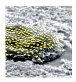
These nanoscale dots contain optical elements and electronics that adhere to individual live cells—a breakthrough that could enable remote tracking of cell health and provide early warnings for disease.
