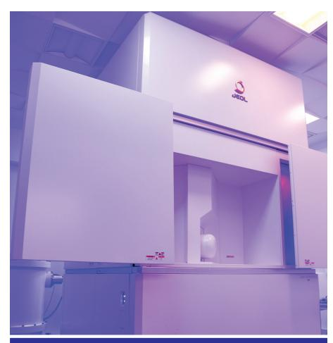
The MCP's JEOL Grand ARM (Atomic Resolution analytical Microscope) II offers subatomic resolution, enabling researchers to explore matter at the scale of less than 60 trillionths of a meter.
