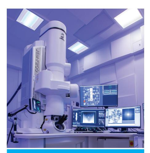
The transmission electron microscope (TEM) uses an electron beam to visualize specimens and generates highly magnified cross-sections of materials.
