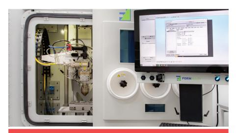
The Directed Energy Deposition machine enables researchers to build bespoke alloys layer by layer, offering unprecedented control over materials design.
