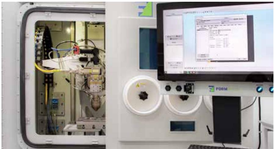
The Directed Energy Deposition machine enables researchers to build bespoke alloys layer by layer, offering unprecedented control over materials design.
