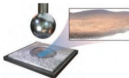
Deposited on rough surfaces, fatty acid layers form contact junctions that explain frictional aging, as was highlighted by cutting-edge research combining friction experiments, molecular simulations, and a theoretical model.
