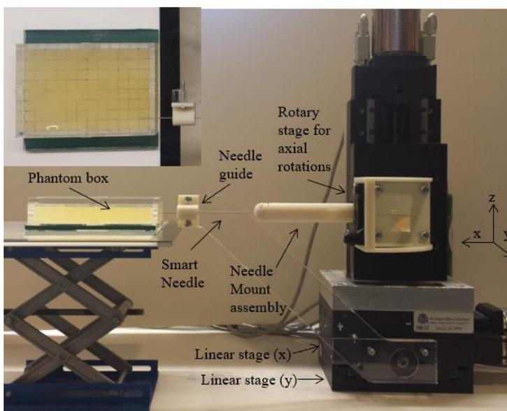
Figure 2: Soft phantom insertion setup
