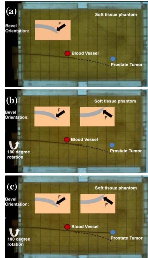
Figure 1: (a) An insertion with the bevel-tip oriented upward and a misaligned needle trajectory. (b) 180 degree axial rotation reverses the bevel angle. (c) The needle is fully inserted to the target.
