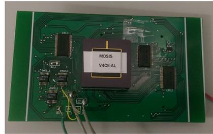
Figure 1: IFAT chip connected to PCB
