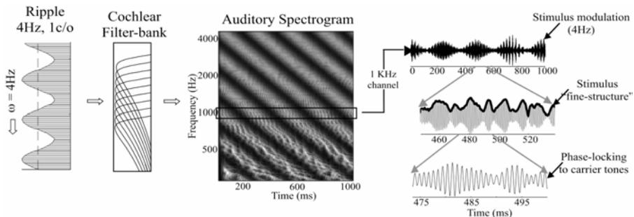
**Fig. 1.** Schematic of stimulus envelope and fine structure. **Left:** A ripple stimulus (4Hz and 1 c/o) is given as input to a filter-bank. **Middle:** The filters outputs show an overall pattern of a 4Hz drifting spectrogram. **Right:** The output of the 1KHz channel reveals the 4Hz envelope modulating a more dense fine structure carrier.
