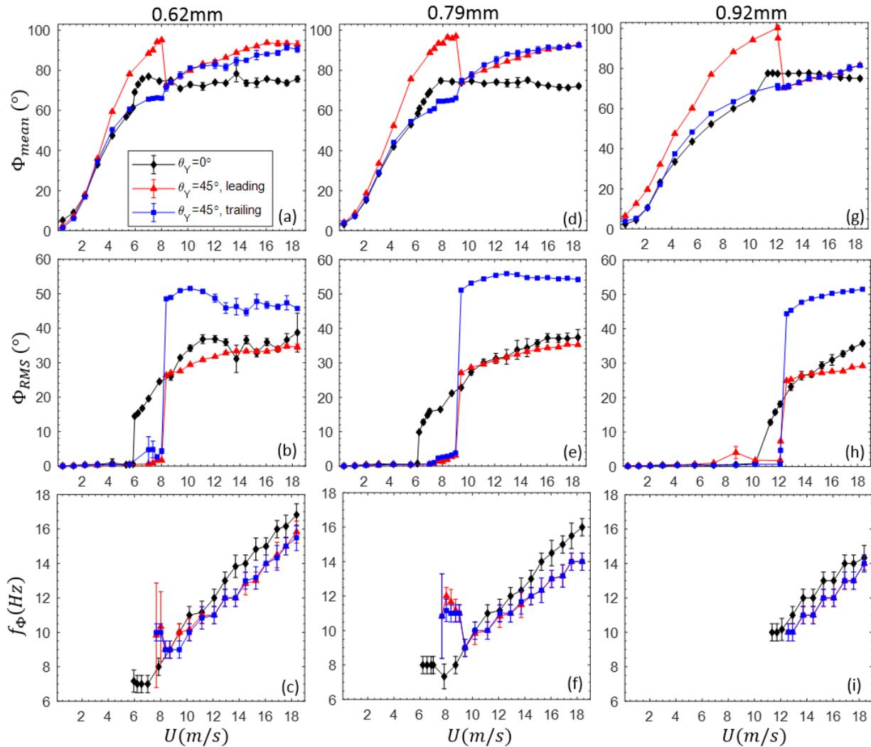
**Figure 6.** Membrane motion with the increase of flow velocity at  $\theta_Y = 0^\circ$  and  $45^\circ$ . (a, d, g), (b, e, h), and (c, f, i) show the mean deflection  $\Phi_{mean}$ , flutter amplitude  $\Phi_{RMS}$  and the dominant frequency  $f_\theta$  of tip flutter, respectively. The standard deviation in the six individual experiments for each case is also shown in the plots.
