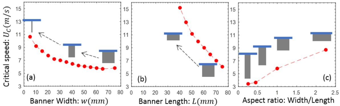
**Figure 7. Membrane critical speed ( $U_c$ ) as a function of membrane shape and size for  $\theta_\gamma = 0^\circ$ . (a) Change with increasing width and fixed length; (b) change with increasing membrane length and fixed width; and (c) change with increasing membrane aspect ratio with fixed area. In these experiments, (a) and (c) use  $0.62 \text{ mm}$  membranes and (b) uses  $0.79 \text{ mm}$  membranes.**
