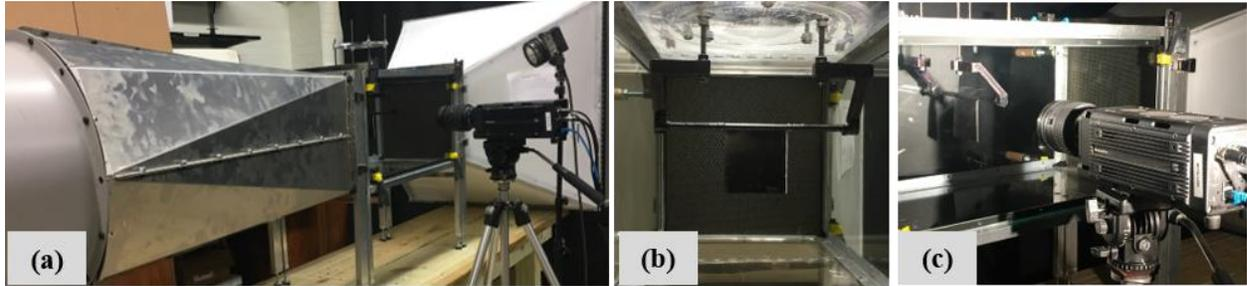
**Figure 2. Experimental setup when Yaw angle = 0°. (a) The low Reynolds number wind tunnel; (b) Silicone membrane coated with black and white at edge, suspended in the test section; and (c) high-speed camera used to record the membrane flutter.**
