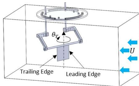
**Figure 1. Schematic of suspended membrane configuration inside the test-section of the wind-tunnel.**
