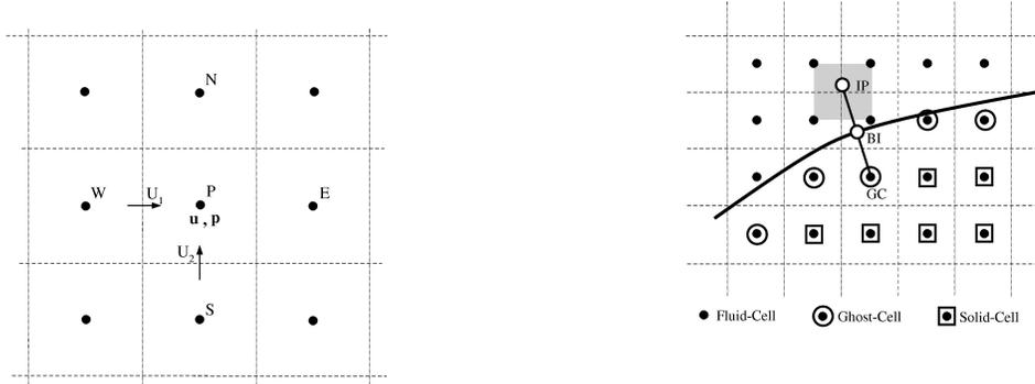
Figure 3. Schematic describing naming convention and location of velocity components (left) and the ghost-cell method (right).
