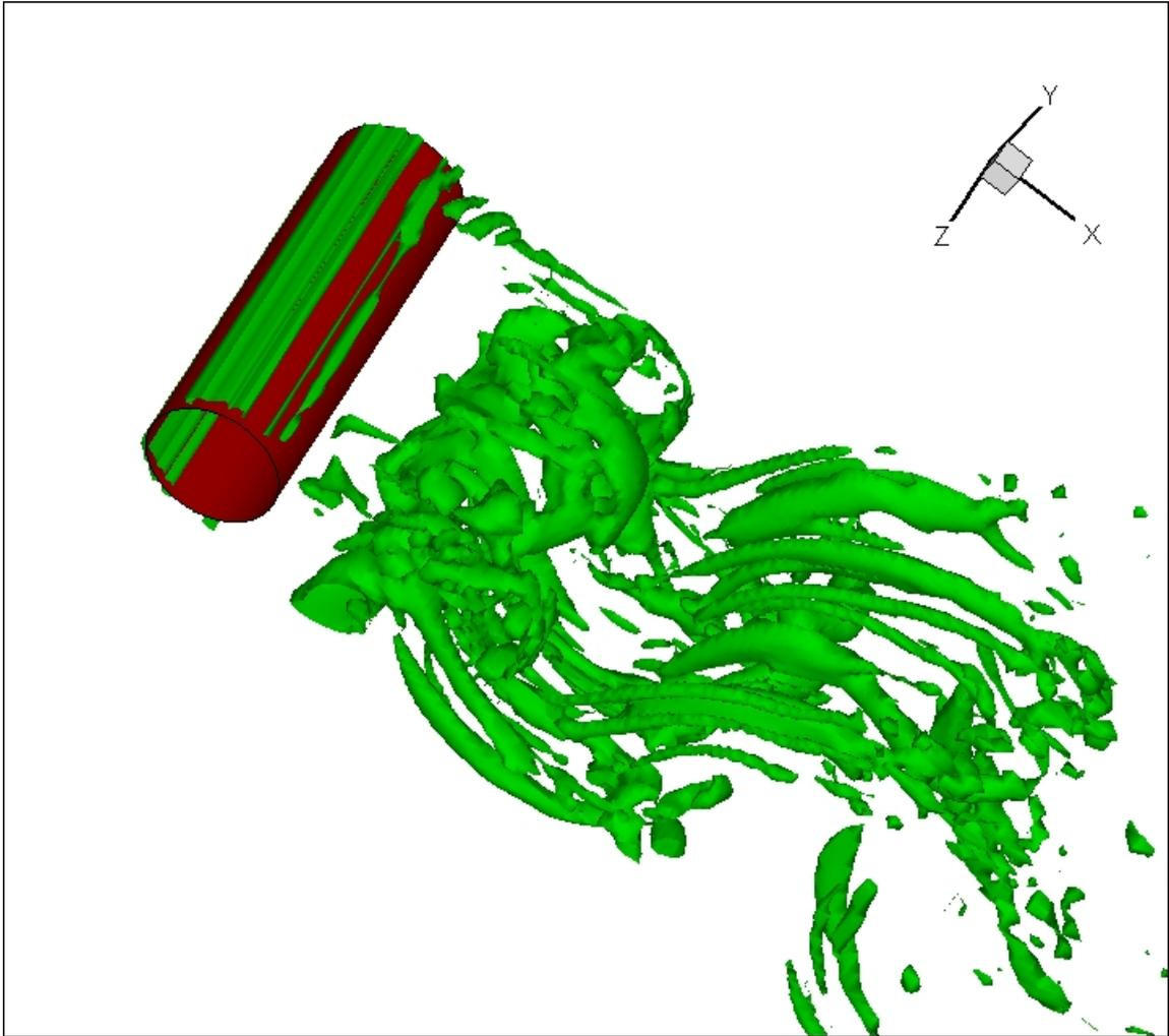
Figure 7. The wake structure of the cylinder.
