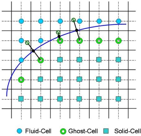
Fig. 1 2D schematic describing ghost-cell methodology
