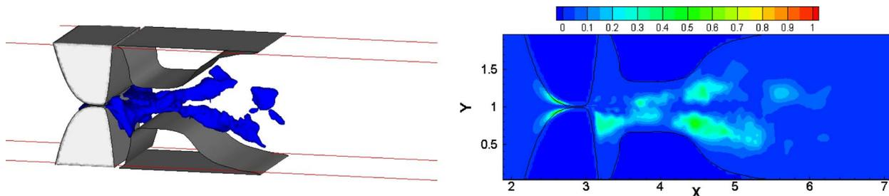
**Fig. 13 Isosurface of the turbulent kinetic energy corresponding to a value of  $K_T=0.15$  and a contour of turbulent kinetic energy at the center plane ( $z=0.75$  cm)**
