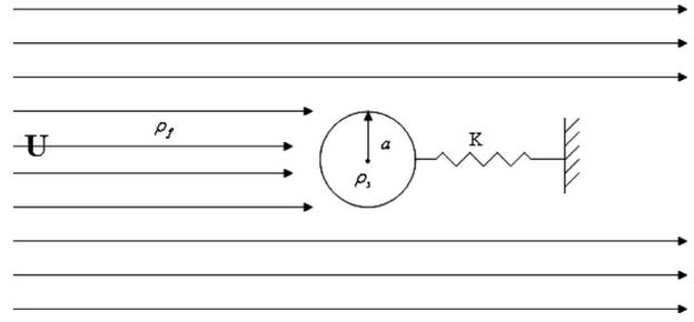
Fig. 3 Schematic flow past an elastically mounted sphere
