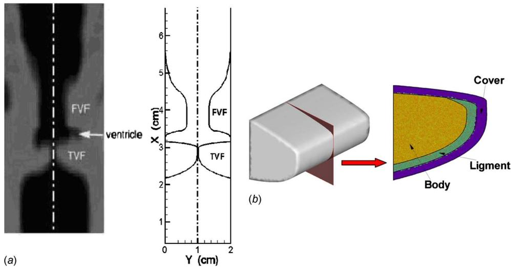
**Fig. 4** (a) A coronal view of CT scan of human larynx and the current flow domain that attempts to match the key geometrical features in the CT scan. (b) Three-layer vocal fold inner structure inside an idealized geometric VF model based on CT scan and triangular elements used in the current solver.
