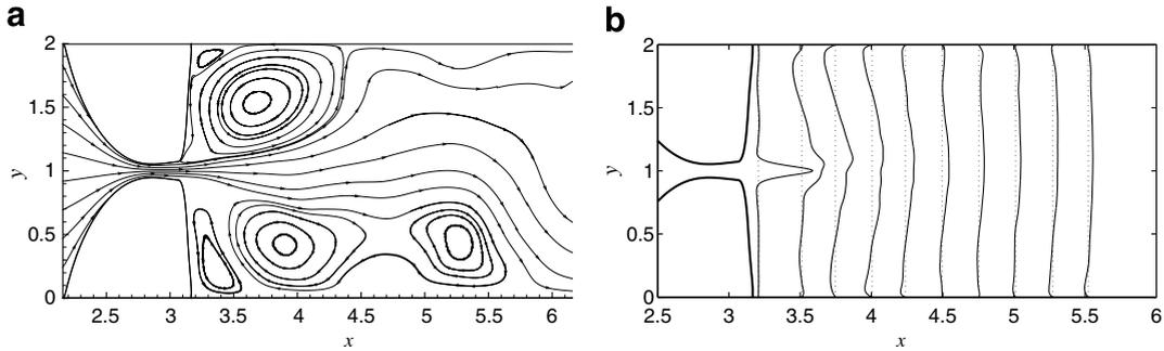
Fig. 22. Averaged flow field between  $t = 18$  cs and  $t = 25$  cs for  $\eta = 10$  p. (a) Streamlines and (b)  $v_1$  velocity profiles at different locations. Every 1 cm represents a velocity of 50 m/s.
