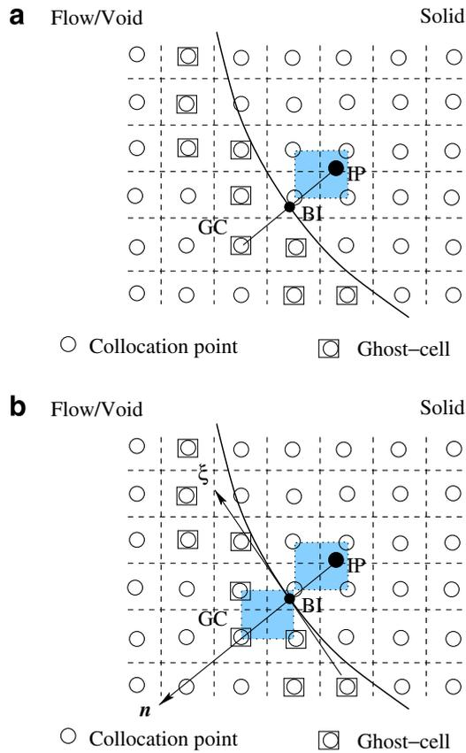
Fig. 4. Schematic of the immersed-boundary method on a Cartesian grid for solving the linear viscoelasticity. The bold curve represents the boundary of the solid. The stencil is shown in (a) for the displacement boundary condition and in (b) for the traction boundary condition.
