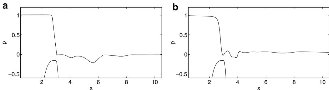
Fig. 19. Gage pressure (kPa) along the centerline of the channel for  $\eta = 10$  p. (a)  $t = 18.20$  cs (closure phase) (b)  $t = 18.40$  cs (open phase). The streamwise position of the vocal fold is also shown.
