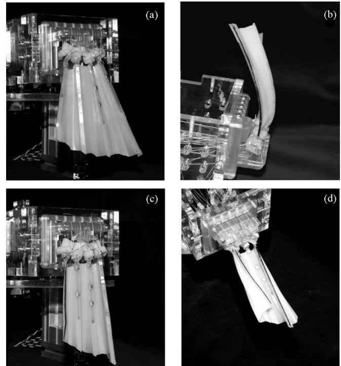
Fig. 10. Component motions: (a) expansion, (b) curl, (c) relaxed, and (d) cupping. Black lines were drawn on the lateral edges of the fin to aid in the visualization of the fin's shape.
