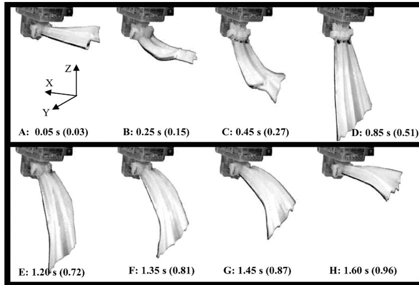
Fig. 12. Images from a video of the four-ray fin conducting a simple sweep motion. The camera angle was from approximately  $45^\circ$  aft of the  $Y$ -axis. The outstroke is shown in panels A–D, and the instroke in panels E–F. The main plane of the fin was aligned predominantly with the  $Y$ -axis during sweep. The time stamp indicates the time within the 1.67-s cycle and the number in parenthesis represents the decimal fraction within the fin’s cycle.
