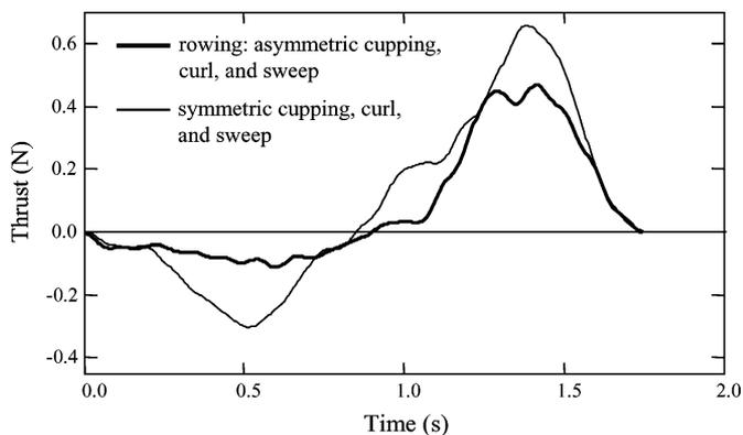
Fig. 16. Forces from the rowing motion. The force created by the fin using sweep, curl, and cupping (thin solid), and when the fin was feathered into the flow during the outstroke by using an asymmetric sweep, curl, and cupping (thick solid).
