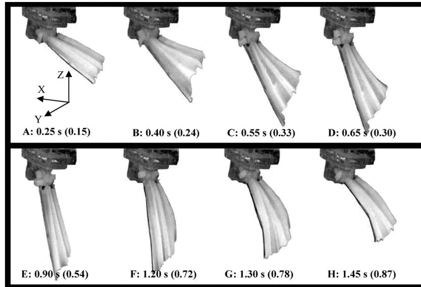
Fig. 15. Four-ray fin conducting a rowing motion. The camera angle is from approximately  $45^\circ$  aft of the  $Y$ -axis. The fin was twisted and feathered into the flow such that its motion was led by the fin's dorsal edge (panels 1–4). The fin was then brought square with the flow (panel 5), such that the main plane of the fin was aligned with the  $Y$ -axis and all fin rays were paddled back together (panels 6–8).
