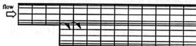
FIGURE 31.1 An example of a flow configuration that would benefit from fully implicit treatment of the momentum equation. Arrows indicate flow in the vorticity direction.
