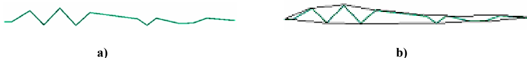
Figure 2. Selected cross-section of a dragonfly wing a) pleated airfoil b) profiled airfoil
