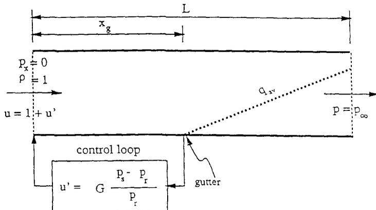
Fig. 1. Schematic of combustor with control loop.
