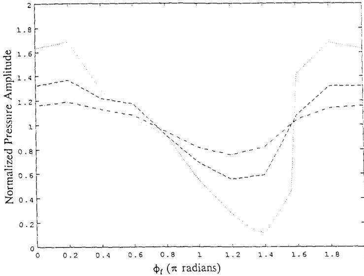
Fig. 3. Variation of peak-to-peak pressure amplitude with phase-lag in feedback (the amplitudes have been normalized with respect to the uncontrolled amplitude).
