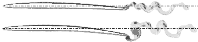
Fig. 8. Sequence of spanwise vorticity contour plots for flow past a flexible foil computed using a Lagrangian vortex method [76], [77].
