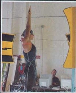
In computational fluid dynamics, a full-body scan of Gabrielle Rose creates a digital model used to analyze water flow around a swimmer.
