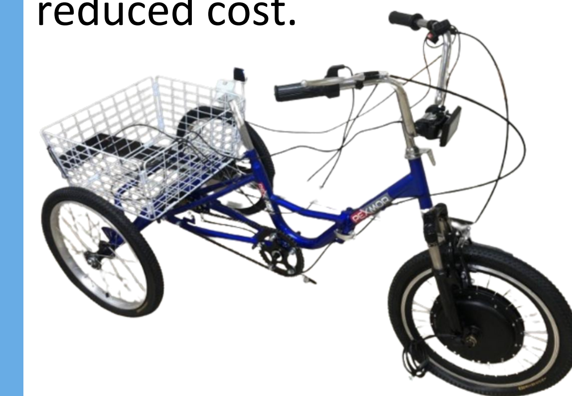
Fig. 4. Partly-Assembled Adaptive E-Trike
