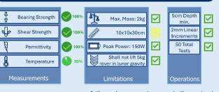
The penetrometer can successfully and accurately record all required data types – temperature measurement accuracy may vary depending on system operation speed. We breached the bounding box vertically, but future models can reduce component size depending on rover dimensions and probe mounting options. The penetrometer exceeded 50 tests in regolith simulant without sensor deterioration.
