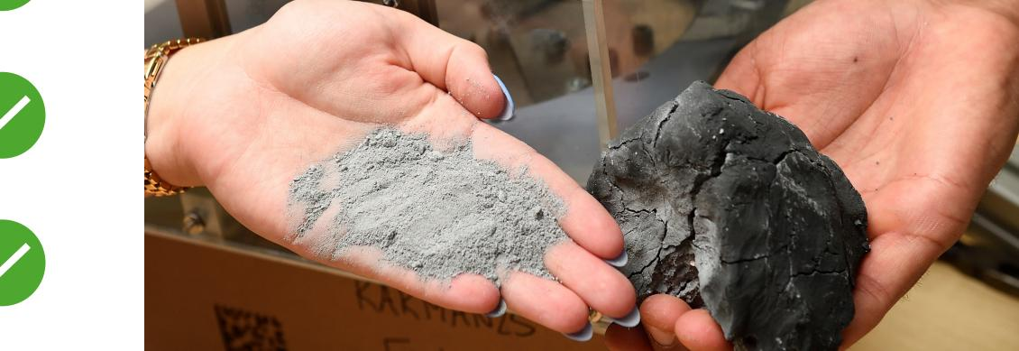
Grinder Subsystem Test: The Grinder subsystem successfully grinds all regolith simulant strengths to below 0.5 mm.
