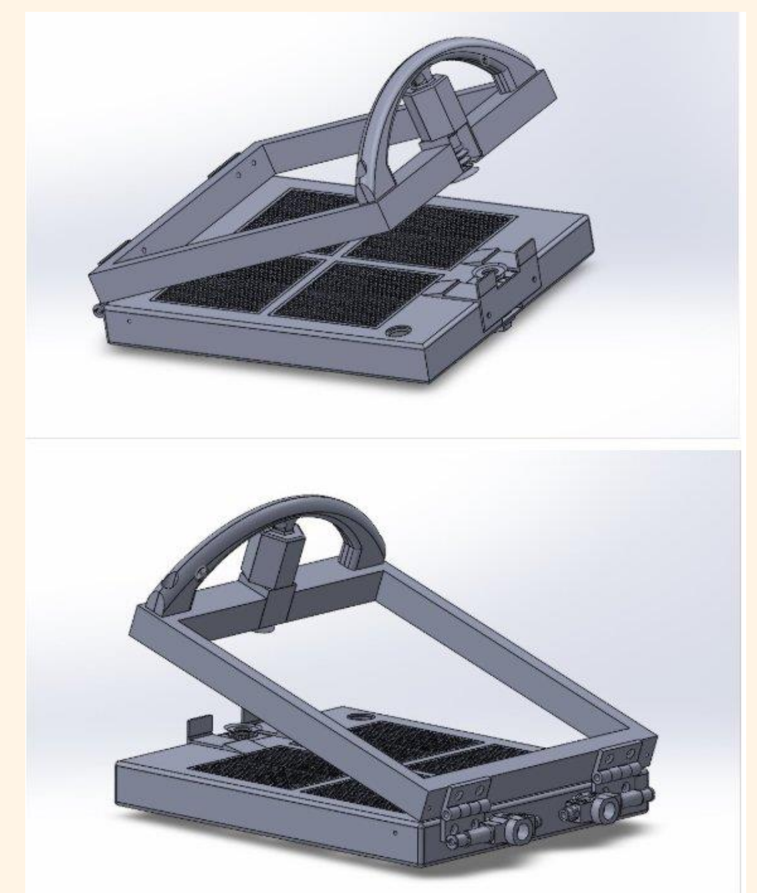
Fig. 3 — Bag opener CAD (closed & open positions)
