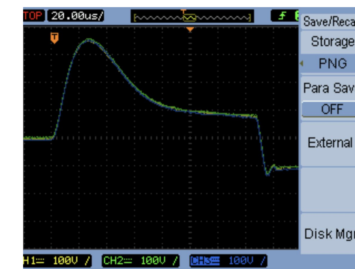
Figure 2A: Oscilloscope screen when reading voltage in channel shows no qualitative difference in signal from the TENS prototype.
