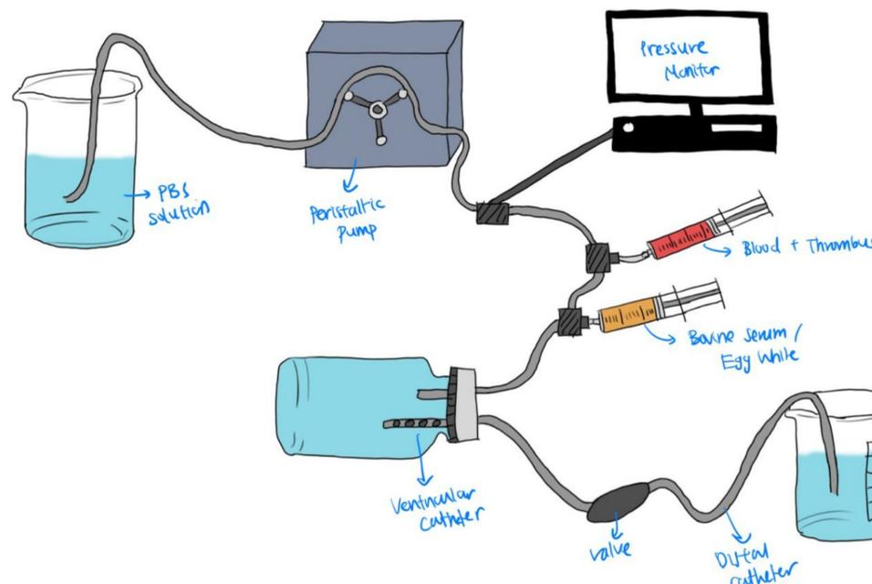
Fig 2. Proposed ventricular obstruction model simulating protein and blood obstruction, with inflow pump and outflow shunt valve.
