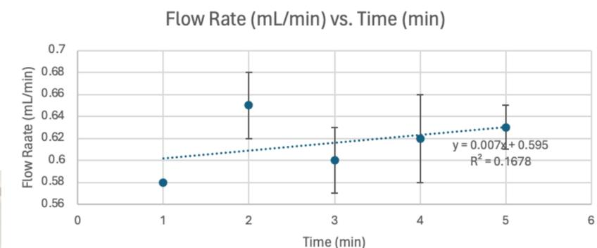
Fig 5. Verification of constant flow through model over five-minute time period.
