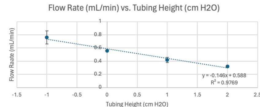
Fig 4. Verification of model to identify tubing height necessary to achieve equal inflow and outflow.
