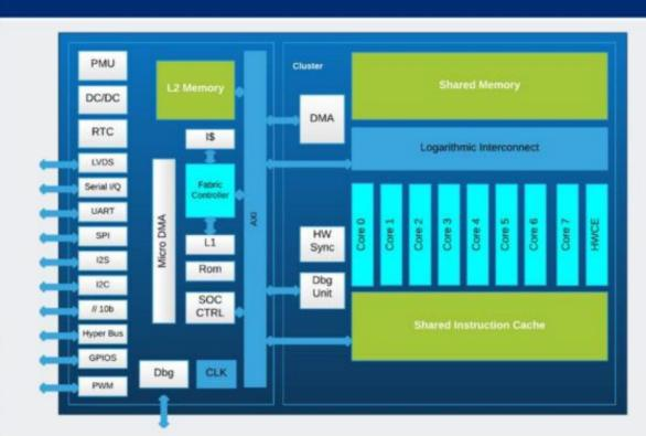
The Al-deck onboarded on the Crazyflie consists of the GAP8 chip developed by Greenwaves Technologies, a parallel, ultra-low-power and flexible RISC-V based IoT application processor for the TinyML ecosystem, which includes MAC (multiply and accumulate) units for accelerating deep learning inference.
