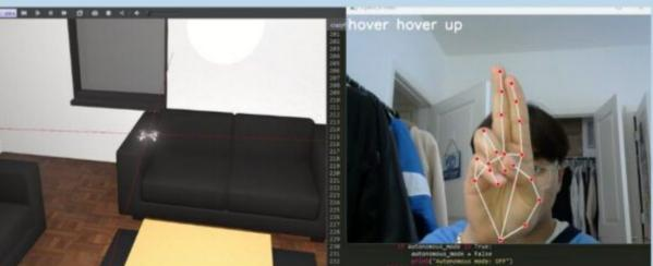
The left half of this screen capture image is the drone in a simulated apartment setting, the right half is the video from the webcam, with the hand features and skeleton overlaid atop along with the predicted gesture.
