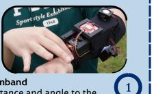
Distance and angle to the basket and the disc are communicated via vibration motors and a speaker. GPS and 2.4 GHz RF enable communication between the armband and the modules
