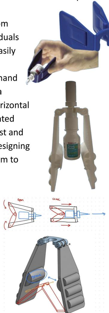
**Fig. 1.** Device Ideation of the Nasal Spray Assist
