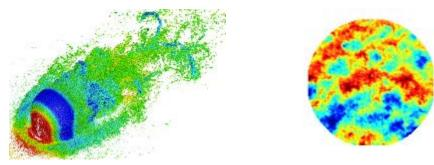
Aero-optics of flow over a hemisphere-on-cylinder turret at Mach 0.4 and  $Re_D = 2.3 \times 10^6$ . Left: vortical structures visualized by iso-surfaces of  $\lambda_2$  colored by density; right: wavefront distortions for an optical beam propagating through a wake region.
