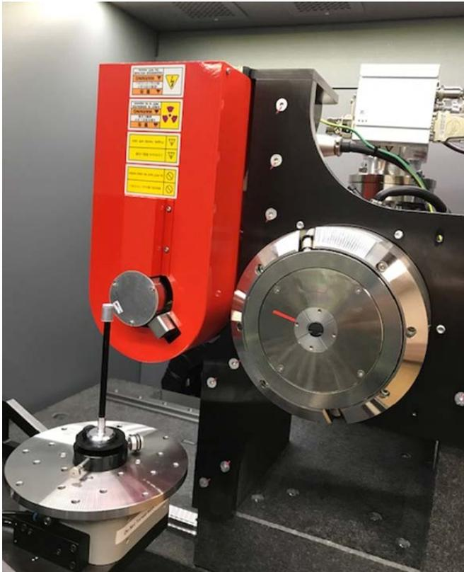
**In this picture the red sealed source has an optional beam filter installed, whereas the silver open source does not have an optional beam filter installed.**
