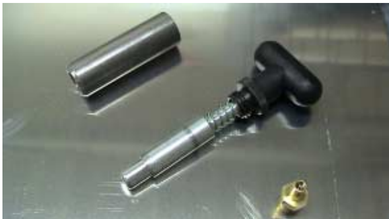
Figure 7.9 – Spring-loaded slider locking pin and brass air pressure release valve
